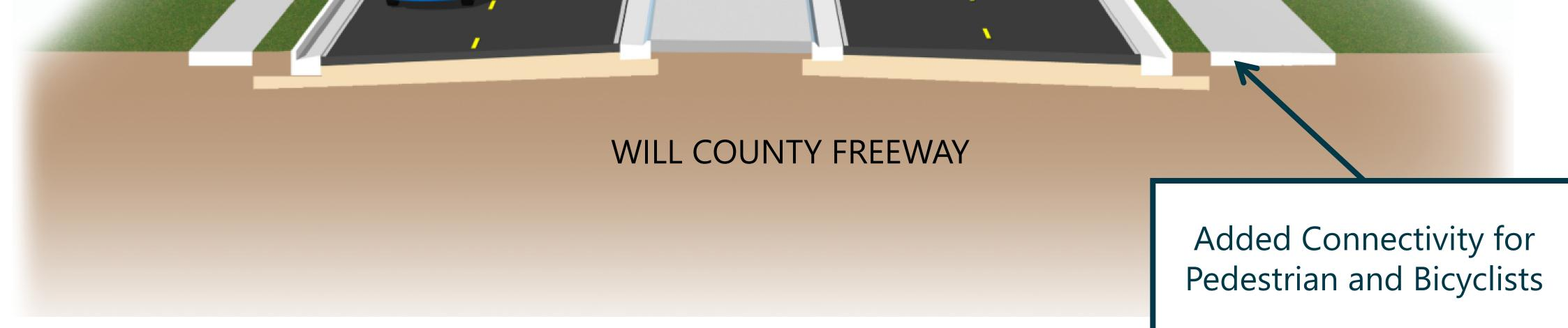
The proposed improvement includes widening Gougar Road to a four-lane roadway with a raised median and curb and gutter. New or upgraded bicyclist and pedestrian facilities will be accommodated on both sides of the road.
